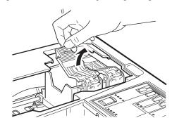
Open the foil ink cartridge packages and remove the cartridges. Then remove the tape seal from each ink cartridge as shown below.
